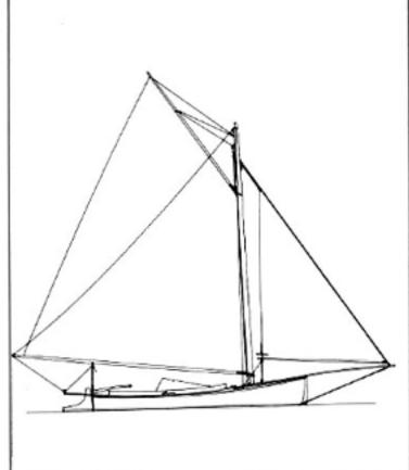
Usually referred to as a sandbagger, SHADOW is a smoothplanked, shoal-centerboard oyster sloop with a reduced cat rig. She was built at Stratford, Connecticut and used as a racing boat. Her design includes a flat stern, good deadrise, hoggeddown bowsprit and oval cockpit. She is typical of a small range of oyster sloop, gaff-rigged, with a rocker to keel bottom. She has two mast steps for either a sloop or cat rig.
