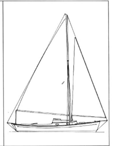
MENEMSHA is a classic shoal-draft singlehander with an unusually large cockpit for daysailing, and cruising accommodations for two or three. A long keel combined with a fine entry, an easy run, and fifty percent ballast ratio give the MENEMSHA an easy motion in a seaway and stiffness in a fresh breeze.
