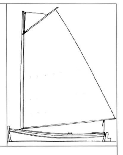
Originally used as a Newport fish and lobster boat, this shallow keel, clinker-built cat boat has a roomy cockpit with a central wet well. When Bob took PEGGOTTY's lines, he was working from a hull design already more than 125 years old. The resulting boat is straight forward and practical, gaff-rigged, but with the simplest imaginable running rigging. A cockpit large enough for eight people makes PEGGOTTY great for daysailing or picnics.
