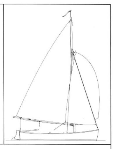
The fiberglass SPIRIT was originally designed for George O'Day and named the SPRITE. (3500 were built) This safe and versatile jib-headed, centerboard sloop features two mast steps, allowing her to be cat rigged for the beginner, then sloop rigged with main and jib for the more advanced sailer. She will carry two adults or three children.
