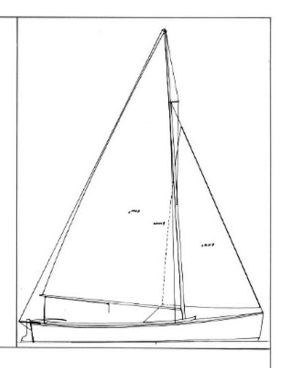
With its long, flat run, the sloop DRAGONFLY is fairly typical of early planing hulls. A clever centerboard mechanism, invented by Bob, allows the board to be adjusted fore and aft to perfect the balance of the boat. DRAGONFLY will carry a crew of two for racing, or five for day cruising. Construction is strip-plank.
