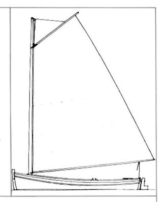
Originally used as a Newport fish and lobster boat, this shallow keel, clinker-built cat boat has a roomy cockpit with a central wet well. When Bob took PEGGOTTY's lines, he was working from a hull design already more than 125 years old. The resulting boat is straight forward and practical, gaff-rigged, but with the simplest imaginable running rigging. A cockpit large enough for eight people makes PEGGOTTY great for daysailing or picnics.
