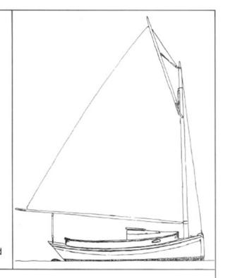
This seakindly catboat with her raking stern and comfortable cabin makes a fine weekender or daysailer. She has a gaff rig, 294 square feet of sail, a full keel and smooth-plank construction. For cruising, two berths are typical, although she will comfortably carry four to six adults.
